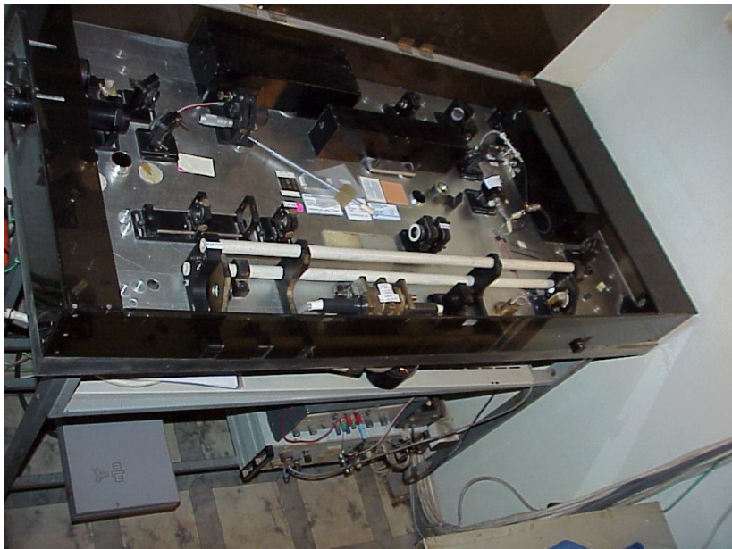
Fig.(4): The Nd:YAG laser transmitter of the Helwan satellite laser ranging station.
