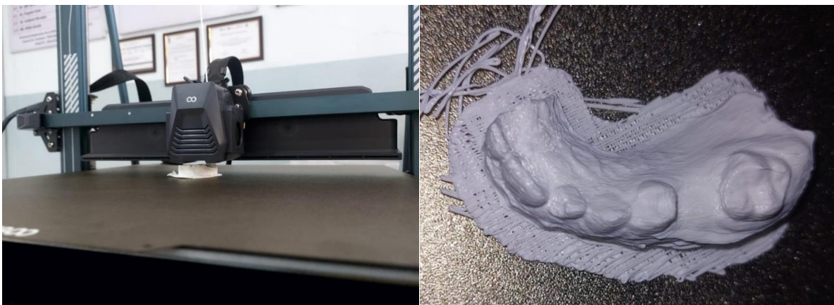
Fig. 3. ELEGOO Neptune 4 plus FDM 3D Printer and 3D model
