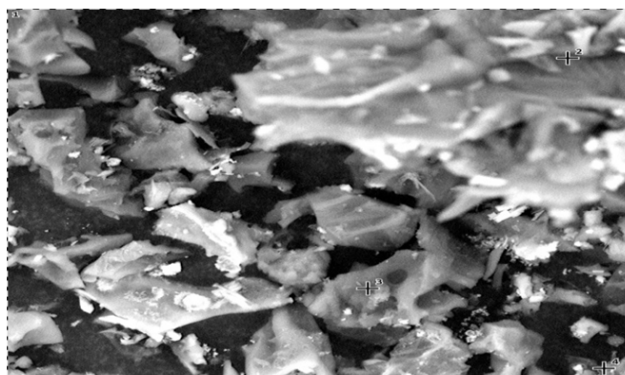
Plate 2. SEM analysis of KNS -AC at 75 \mu\text{m} particle size (Mag.= 5000x)
