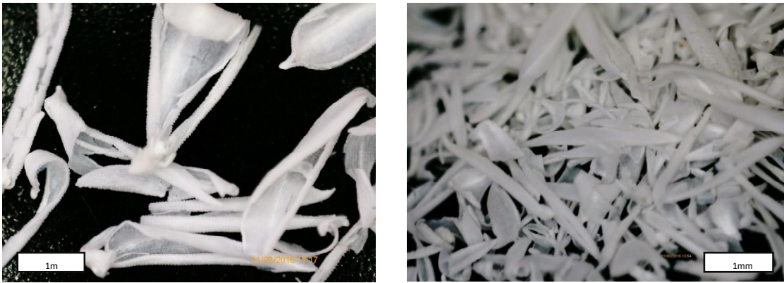
Fig. 3. Close observations of rice husk ash (a: left) in individual and (b: right) in a flock
